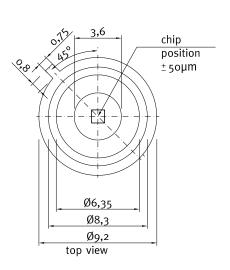
UVC-only SiC based UV photodiode A = 1.00 mm<sup>2</sup>
